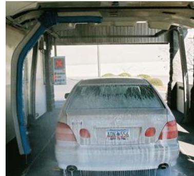
**Foaming Presoak 2** applies a different formulated soap to remove stubborn soils and grime that are unlike road film.
